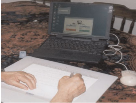
Figure 1. The computerized system, including laptop computer, ComPET software, and digitizing tablet.
